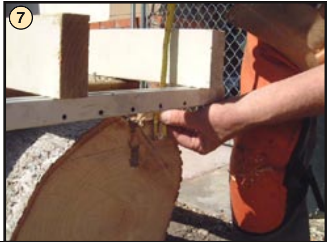
6 Measure down from the top of the 2 x 4 and determine the location of your first cut. If your log tapers you will be cutting a thicker slab at the large end of the log. Try to cut the smallest possible slab on this first cut. Make sure you lower the mill enough to miss whatever toe nailing you may have done.
