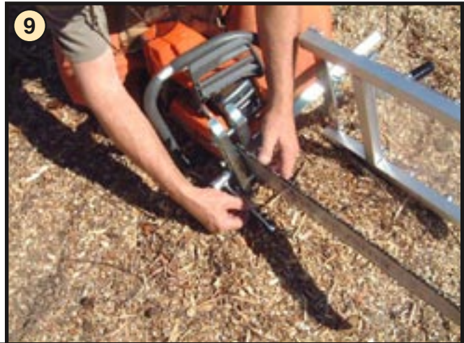
8 Attach the Small Log Mill to your saw as shown. Make sure clamping bolts are equally spaced from the center of the bar. Tighten to 10 to 12 lbs. of torque.
