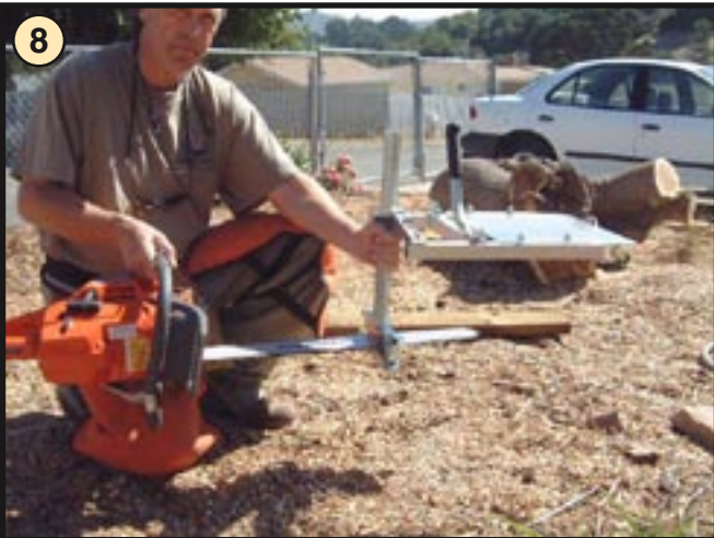
8 Attach the Small Log Mill to your saw as shown. Make sure clamping bolts are equally spaced from the center of the bar. Tighten to 10 to 12 lbs. of torque.
