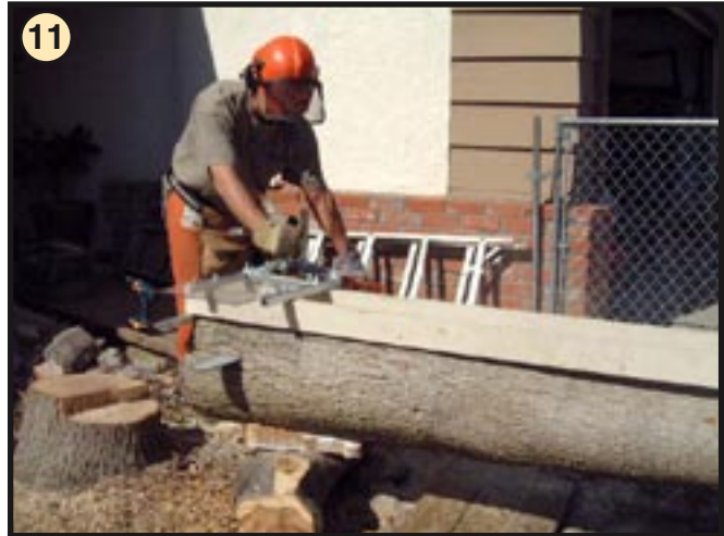
11 Set mill on guide rails and make your first cut. Push the mill evenly through the wood keeping the mill guides down on the 2 x 4's. Use a small wedge and insert in saw cut when you have cut approximately half of the slab. Keep the mill level when exiting the cut.
