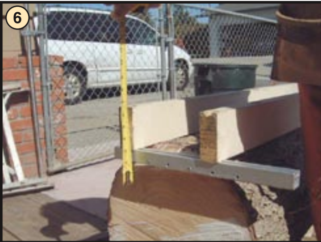
6 Measure down from the top of the 2 x 4 and determine the location of your first cut. If your log tapers you will be cutting a thicker slab at the large end of the log. Try to cut the smallest possible slab on this first cut. Make sure you lower the mill enough to miss whatever toe nailing you may have done.
